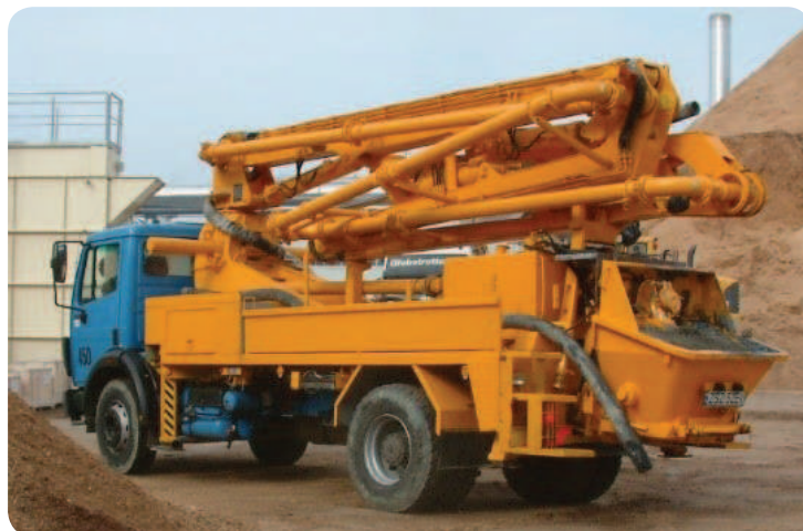
Gambar 2.6 Concrete pump Sumber: Radomil/commons.wikimedia.org (2006)
