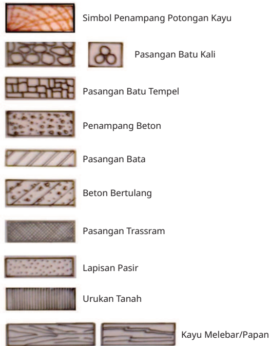
Gambar 4.22 Macam-macam arsiran gambar teknik bangunan Sumber: Kemendikbud/Saelungun Sinaga (2017)
