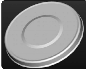
Fig. A5.4 Top Half of the Container after Performing Operations Like Embossing of the Top Surface and Curling of the Edges
