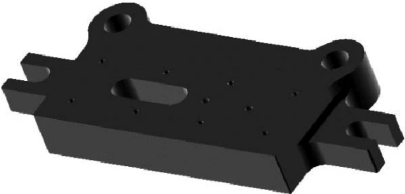
Fig. A4.10 Solid Model of the Bolster Plate-Progressive Die
